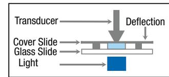
In this test, samples were exposed for 60 seconds to a 3M™ ESPE™ Visilux™ 2 Visible Light Curing Unit. The final shrinkage was recorded 4 minutes after the end of light exposure.
