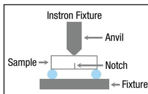
This is similar to 3-point bend (similar to the fixture that provides flexural strength and modulus data).
