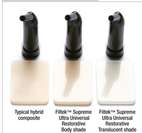
Figure 4: Side-by-side photos comparing composite surfaces after 6,000 cycles of toothbrush abrasion.
