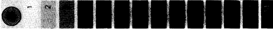
Fig. 41. A value scale: A range of grays from black to white used to gauge gray tone in photography.
